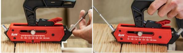
Attach the Torx bit in a drill and drive the screws into the material until the wider part of the bit rests on the guide. Release the jig from the decking board using the red lever and secure it at another spot.
