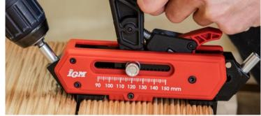
The joint should be a minimum of 25 mm from the edge of the board.
