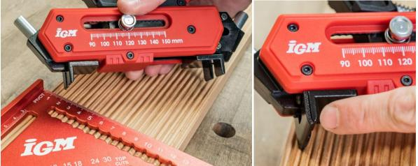
Clamp the jig to the board by pushing on the handle. Insert decking screws into both guides.
